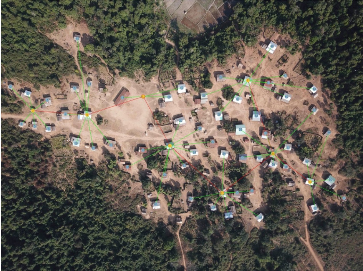
Figure 6: Automated mini-grid design based on drone map of Thapaiban
