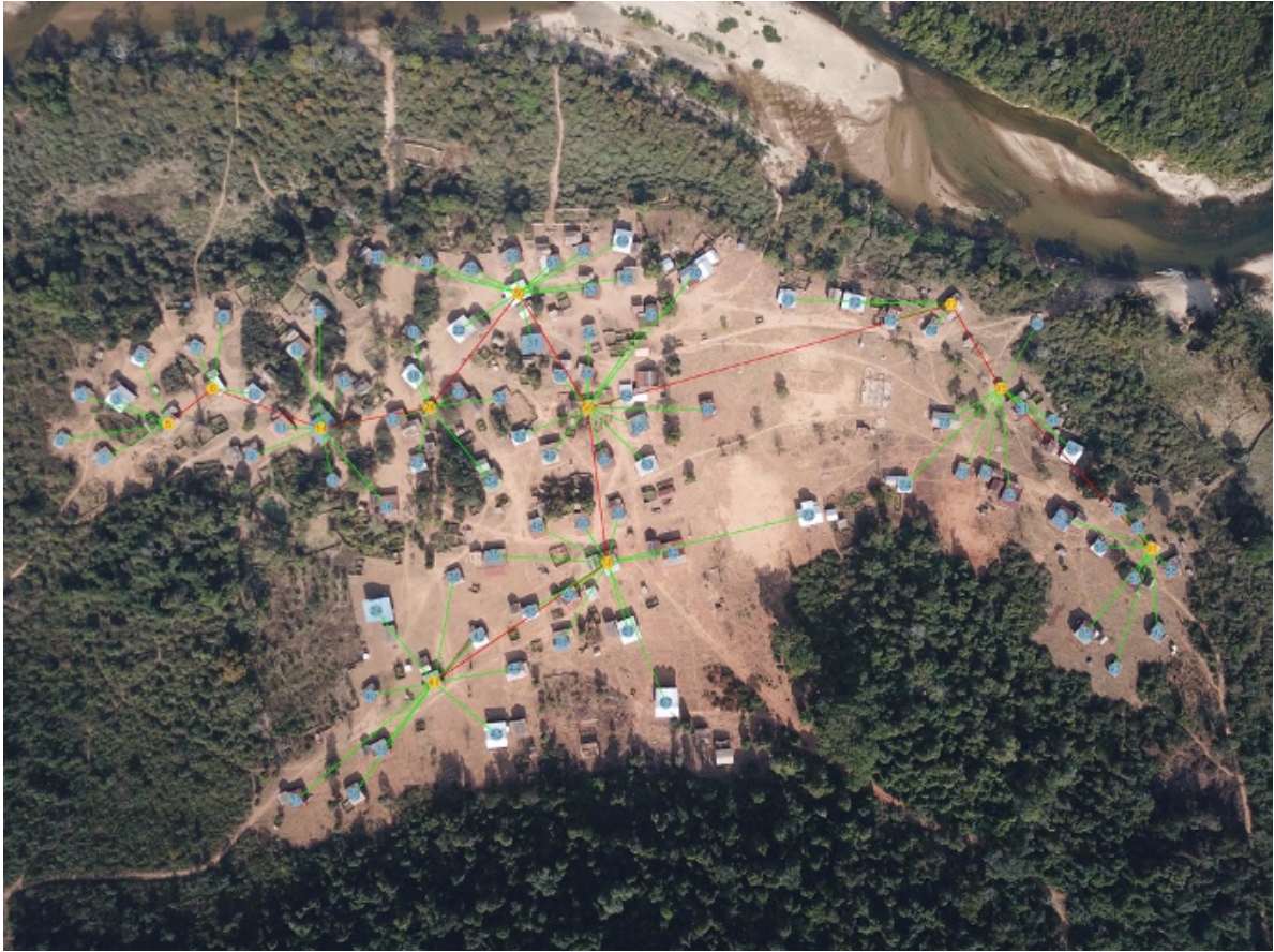
Figure 5: Automated mini-grid design based on drone map of Kobong
